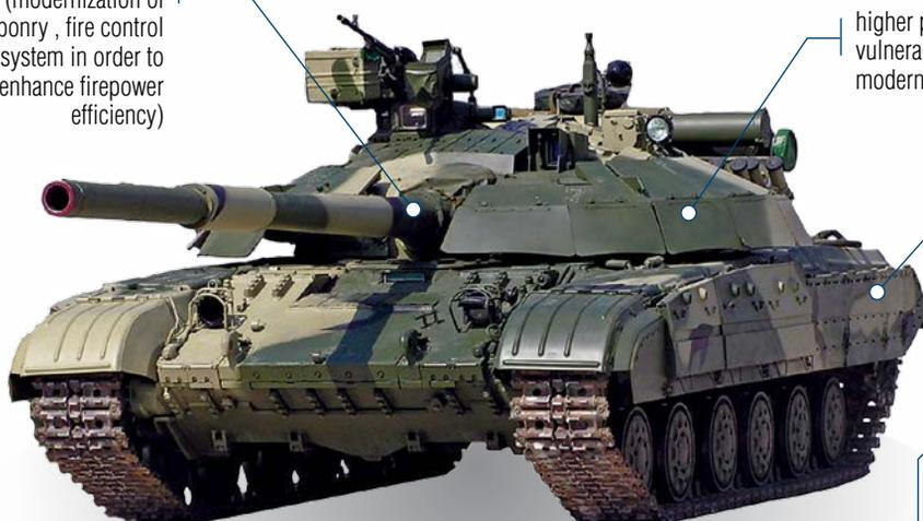
In order to enhance the mobility the power unit of higher power capacity is installed in the engine transmission compartment. The 850 horsepower 5TDFM Engine, being a deeply modified 5TDF Engine version after conduction of power increase measures, is to be used as a new power unit.
